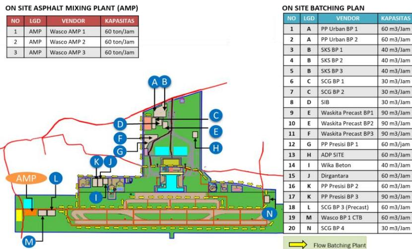
**Figure 5. Location Map On-Site Batching Plan**
