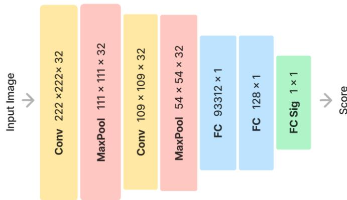
Figure 5: The native CNN architecture used in this research for binary classification of granulation process images.
