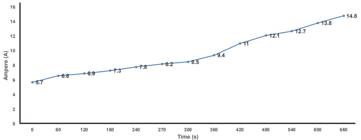
**Fig. 7 : Ampere recorded during the granulation process.**
