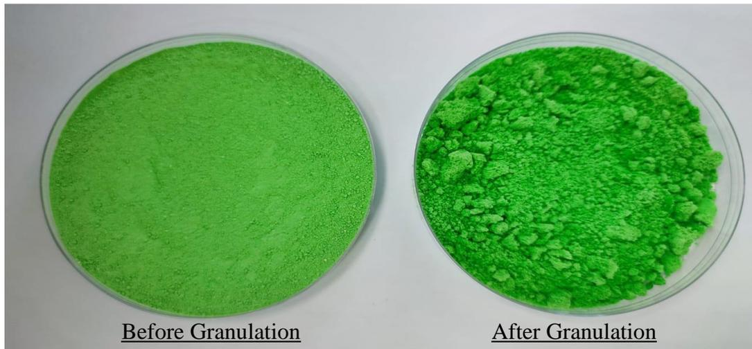
**Fig. 6: Sample of images captured before and after the granulation process.**
