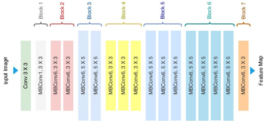
Fig. 4 The EfficientNetB0 architecture
